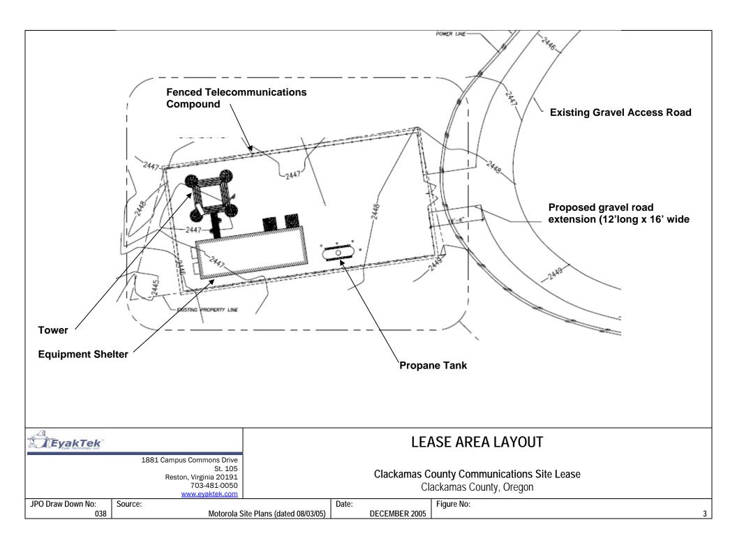
**Tower Design Features** (See Figure 4): Below are the general design features of the proposed telecommunications tower.
